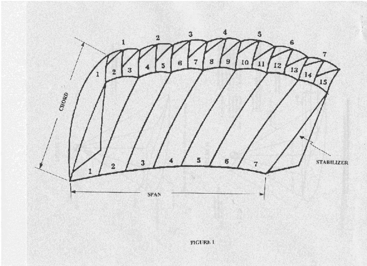
LOADED RIB WITH DIRECTLY ATTACHED SUSPENSION LINES SHOWING SUSPENSION LINE MEASUREMENTS AND TRIM DIMENSIONS
